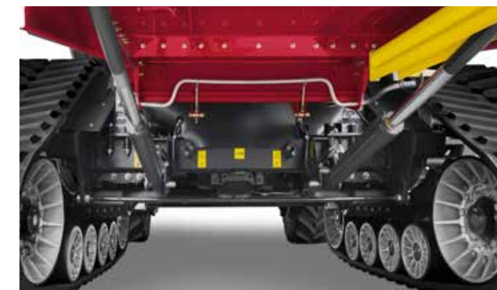
Repositioned lift cylinders for higher lift capacity. Dual lift cylinders for improved header height control
