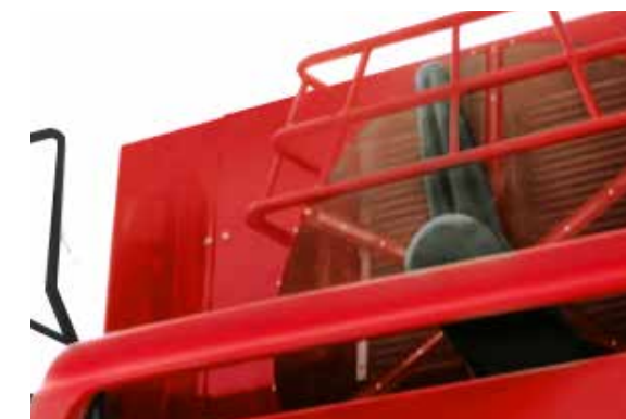
Fixed radiator grille for optimal dust clearing
