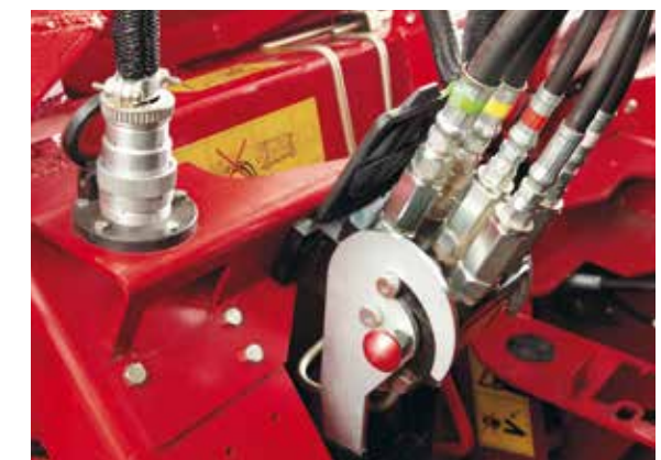
Mount the header in a matter of minutes with the single latch that connects all hydraulic and electric services
