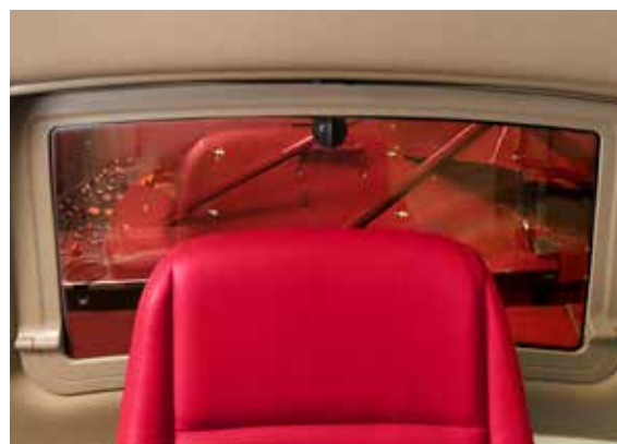
Large inspection window behind operator's seat
