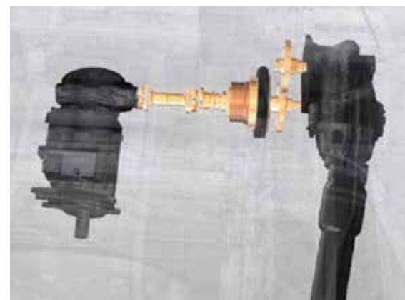
Compact beltless rotor drive with three-speed gearbox for slow speeds in sensitive crops
