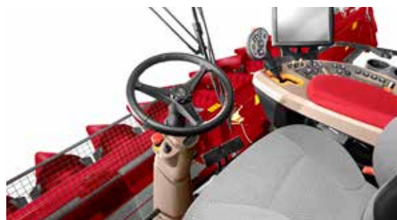
Foldable steering column with new emergency switch and telescopic extendable steering wheel - no obstruction to the view
