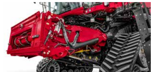
Fore-aft tilting for setting of header angle – all laid crop picked up, minimal losses
