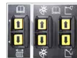
Easy adjustment of the chopper speed or switching from spread to swath via an outside button from the side of the combine
