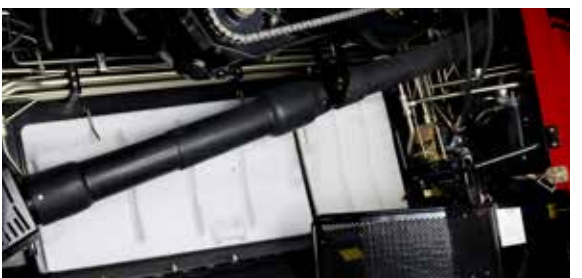
Power Plus drive transfers high power to the feed elevator and header. Simple, low-maintenance design
