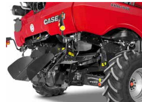
Straw spreader with different spreading options with spread widths up to 14 m
