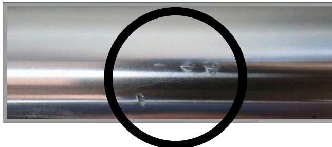
PISTON ROD DAMAGED, POSSIBLE LEAKS
