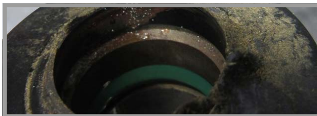
PISTON WITH PARTICLE CONTAMINATION
