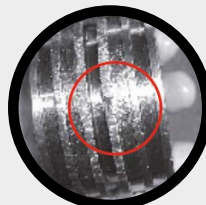
DAMAGE TO THE PUMP PISTON
